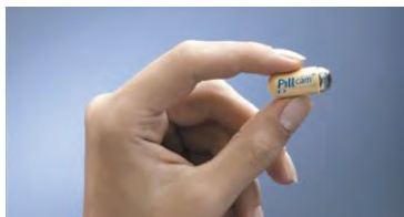
Pill-Cam™, the camera in a pill for diagnosing intestinal disease, invented by Israel's Given Imaging
