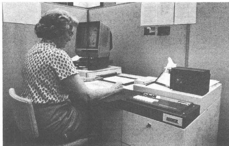
MICROFICHE PROCESSOR — Shirley Rhoades of Editorial Services copies Church publications onto microfiche, a process similar to photocopying. Transferring the Church's major publications to microfiche results in a 90 percent reduction in storage-space requirements. [Photo by Craig Clark]
