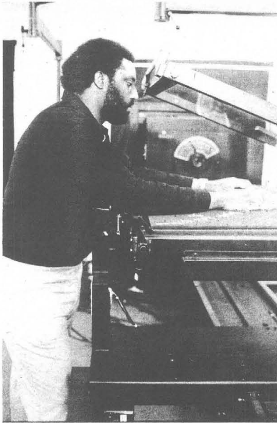
FINAL STAGES — Jerry Frazier, left, arranges a camera-ready layout to make a film negative; Dale Machi uses a magnifier to line up yellow, red, blue and black negatives in film assembly; and Phil Anderson inspects the finished product printed on a two-color Heidelberg PerfeCTOR press. [Photos by Scott Smith]
