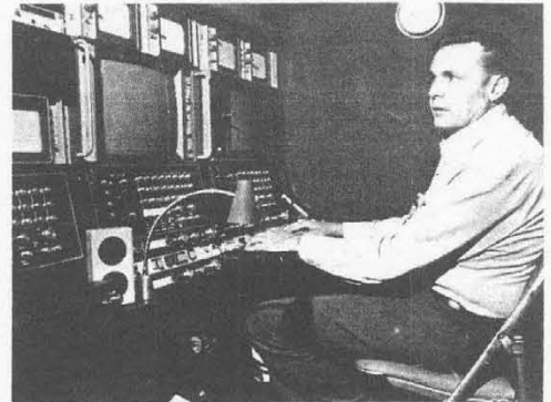
VIDEO POD — Lee Pettjohn, video controller for television production, monitors camera inputs in the video pod during the taping of Garner Ted Armstrong's Kansas City, Mo., campaign of Oct. 17 and 18. The video pod is a portable video-production unit that can be airfreighted anywhere in the world. [Photo by Scott Moss]
