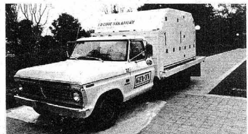
TELEVISION UNIT — The "video pod," a completely self-contained videotape unit that can be airfreighted anywhere in the world, was designed by Ambassador College. The unit is normally carried on a one-ton flatbed truck.
