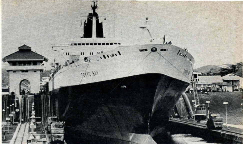
THE TOKYO BAY , shown here and on page 21 at left, the largest ship ever to transit the Panama Canal. The giant container-carrier had only two feet to spare on each side within the 110-foot-wide chambers.
