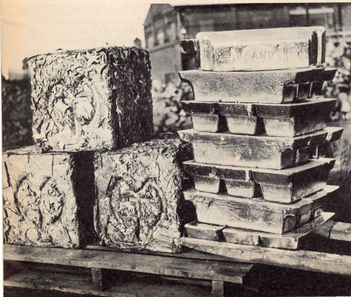
Valuable steel (on left in photo) and tin bars are recovered by M&T Chemicals Inc. The steel can be used by steel mills. Tin is converted into solder or strategic chemicals.
